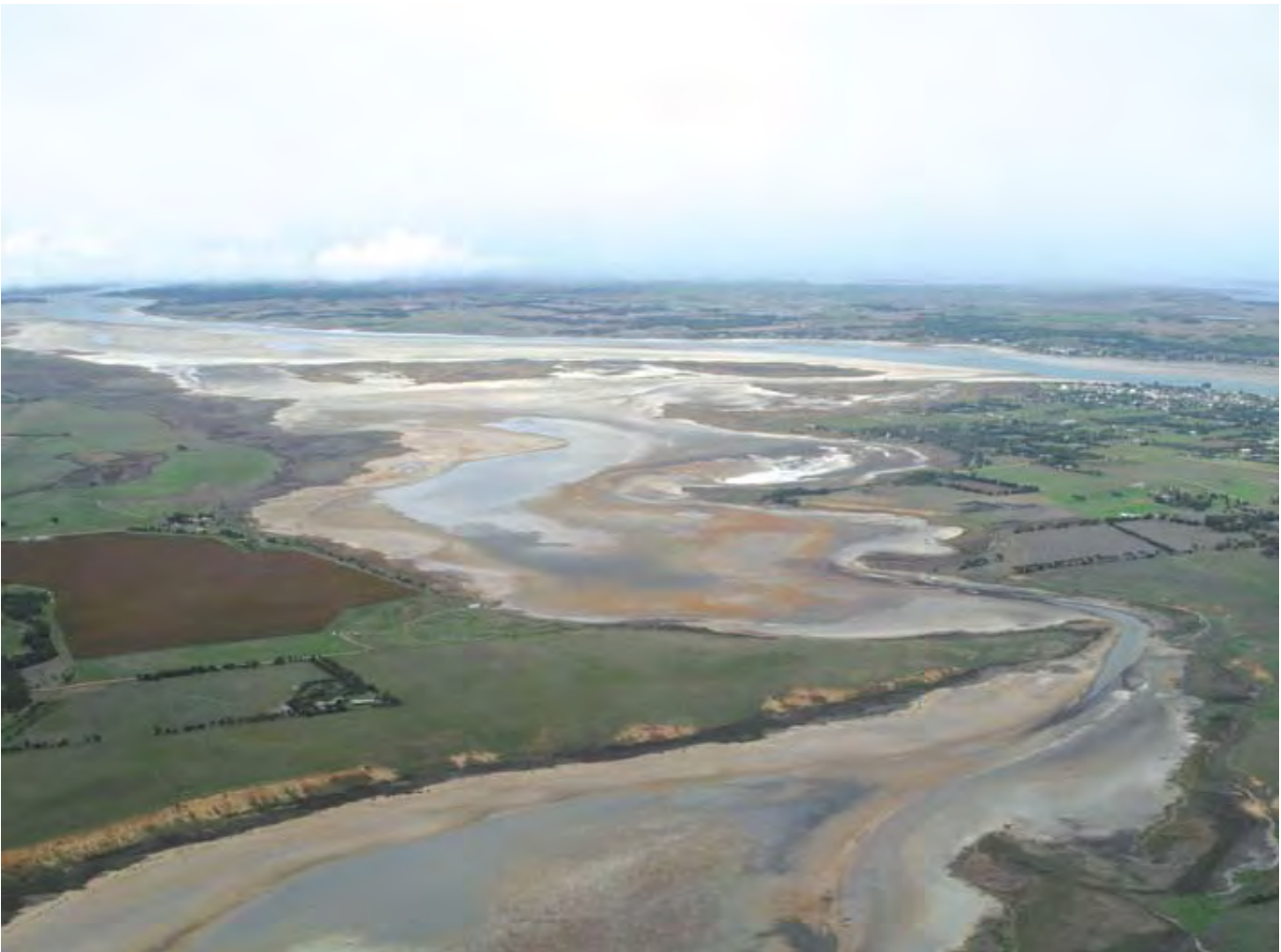
FIGURE 2 ACID SULFATE SOILS (SHOWN BY THE ORANGE TINGE) ACIDIFIED AFTER SEDIMENTS WERE EXPOSED TO THE AIR. THIS IMAGE SHOWS CURRENCY CREEK IN 2009, LOOKING EAST TOWARDS THE LOWER REACHES OF LAKE ALEXANDRINA.
